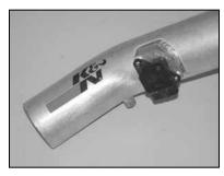
19. Install the mass air sensor into the K&N<sup>®</sup> intake tube as shown using the provided hardware.
