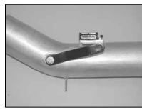
22. Install the provided tube-mounting bracket onto the K&N<sup>®</sup> intake tube with the provided hardware as shown.
