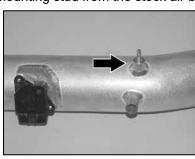
21. Install the engine cover-mounting stud into the  $K\&N^{\text{@}}$  intake tube as shown.
