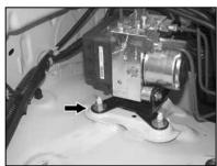
15. Remove the ABS pump mounting nut shown. NOTE: This nut will be reused. Some vehicles may not be equipped with the ABS pump.
