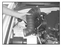
5. Remove the intake tube from the vehicle as shown.
