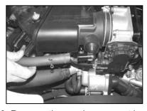
8. Remove the crank case vent hose from the air box as shown.
