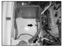
16. Install the heat shield onto the vehicle and secure with the provided hardware and the nut removed in step #15.
