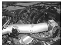
23. Install the K&N® intake tube assembly onto the throttle body and align the tube-mounting bracket with the threaded boss on the valve cover; secure with the provided hardware as shown.
