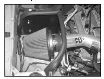
28. Install the  $K\&N^{\otimes}$  air filter onto the intake tube as shown.
