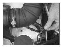
4. Pull the wire harness clip up to release it from the intake tube.
