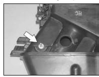
20. Using a 4mm socket, remove the engine cover mounting stud from the stock air box.
