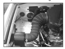
3. Loosen the hose clamps at the air box and resonator.
